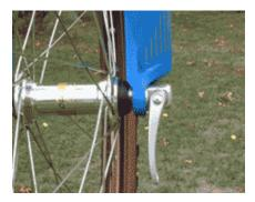
With the wheel centered in the fork (or frame), adjust the quick release by opening it, holding both ends and turning one clockwise until, when you close the lever, you feel some resistance. At this point, try to close the lever. The adjustment is correct when you can fully close the lever but with some effort (the lever should leave its impression in the palm of your hand). If you can only close the lever part way, open it, unscrew the adjustment slightly and try again.
