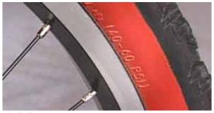
Find the proper tire pressure range on your tire's sidewall.
