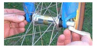
Most forks have wheel-retention tabs on them, which are small protrusions that keep a loose wheel from falling out of the dropouts. The quick release must be open and adjusted by unscrewing to clear these tabs when you remove and install the wheel.
